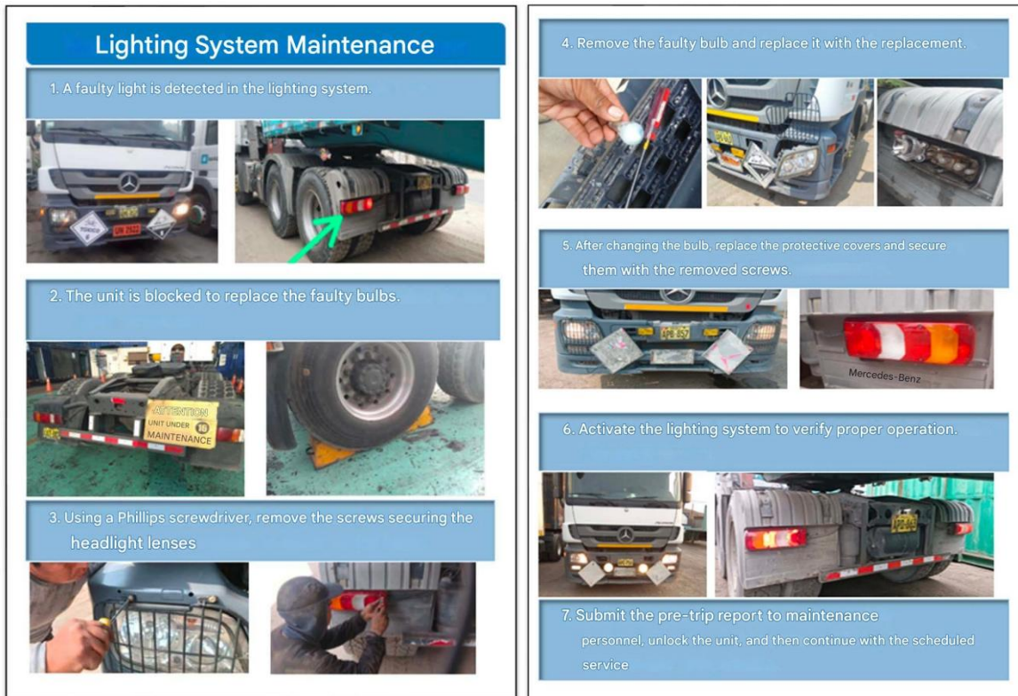
Fig. 6. Instruction for changing spotlights in trucks
